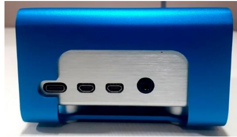
Side-1: RPI Power, HDMI connectors.
